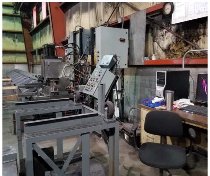
Steel members are factory punched with the highest accuracy to allow for easy bolt-together installation in the field.
