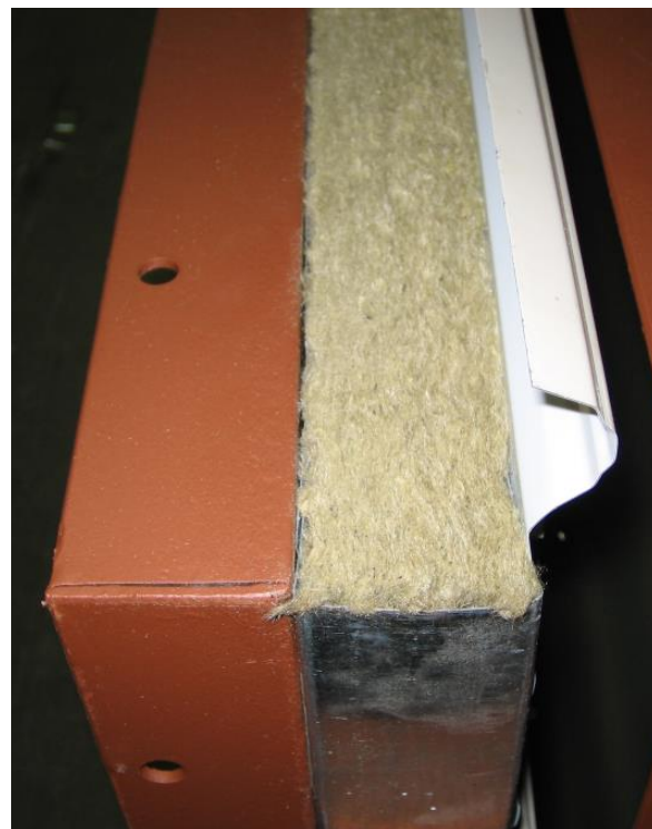
Panel with Mineral Wool Insulation
