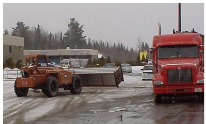
Rack of Panels Being Moved by Telehandler
