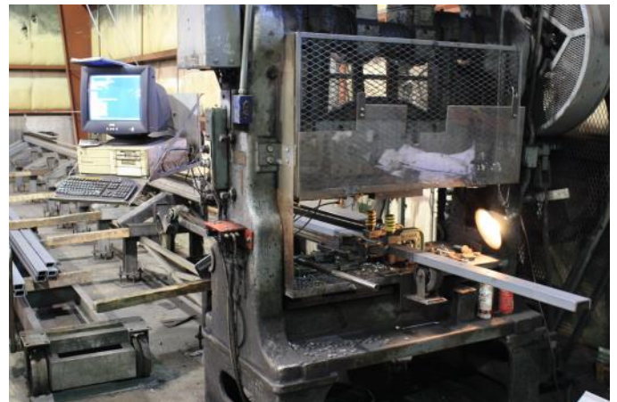
Steel members are factory punched with the highest accuracy to allow for easy bolt-together installation in the field.
