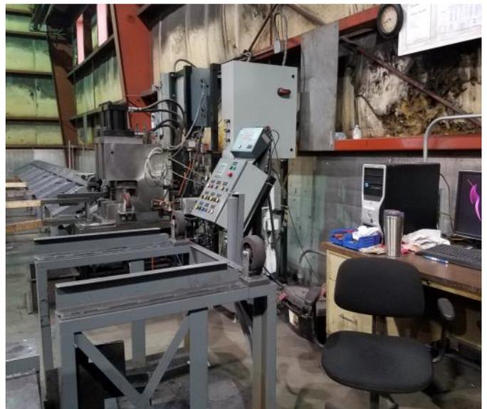
Steel members are factory punched with the highest accuracy to allow for easy bolt-together installation in the field.
