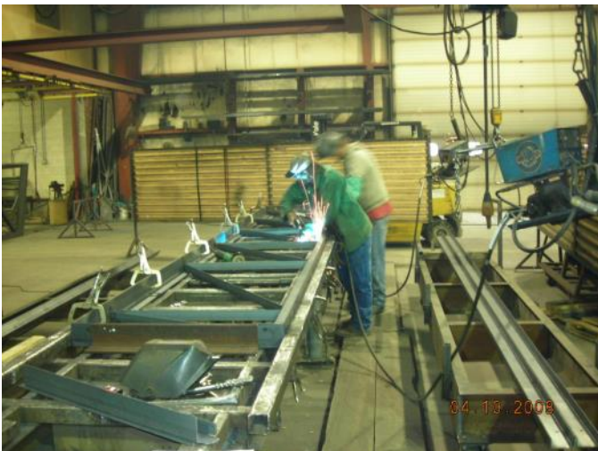
Panels are welded in precise jigs by certified welders to ensure dimensional quality and structural strength.
